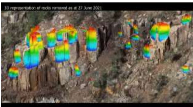
Rocks stacks designated for removal from above the Tasman Highway in Paradise Gorge (image from https://www.youtube.com/watch?v=sITxcv7Ruas )
