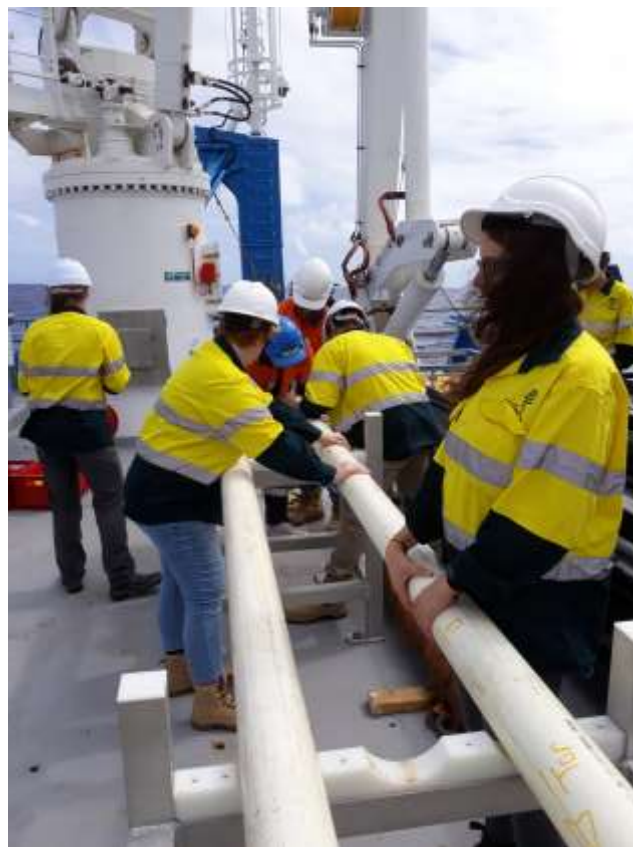
Piston cores on deck of the RV Investigator ready to be extruded (Photo K. Orth).
